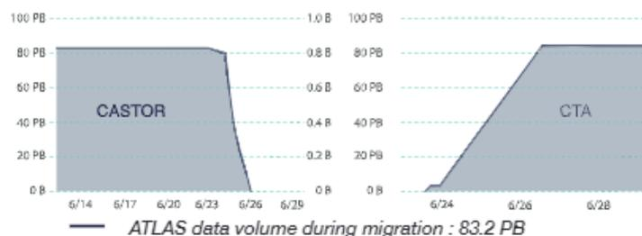
*On 29 June, the CERN Tape Archive (CTA) officially entered production after 83 petabytes of ATLAS data initially stored in CASTOR were successfully migrated to CTA.*
