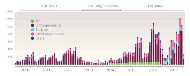
This plot shows on a monthly basis the amount of data recorded on tape generated by the LHC experiments, the other experiments, various back-ups, and the users. In 2017, 72 petabytes of data in total (among which 40 petabytes of LHC data) were recorded to tape with a record peak of 12.3 petabytes in October 2017.
