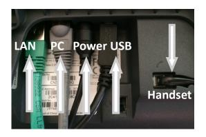
Lan: network cable from a network outlet PC: network cable connected to your PC/MAC USB: cable plugged to a Windows PC (optional) Handset: cable plugged to the handset
